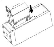
**2** Disconnect the battery wires.
