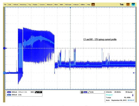
Figure 4. 3TB Typical 12V startup and operation current profile
