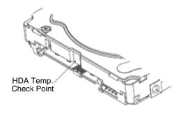
Figure 9. Location of the HDA temperature check point
