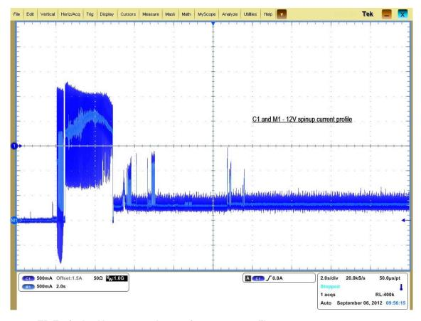
Figure 8. 1TB Typical 12V startup and operation current profile
