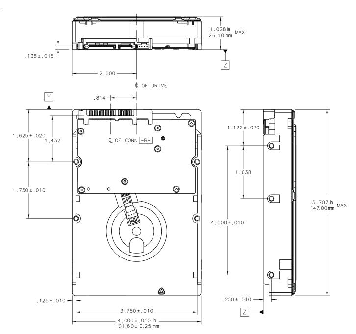
Figure 11. Mounting dimensions—top, side and end view
