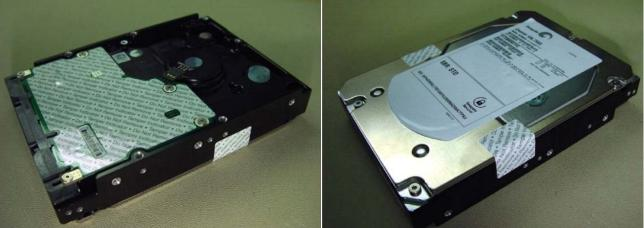
Figure 12. Example of FIPS tamper evidence labels.
