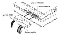
Figure 10. Attaching SATA cabling
