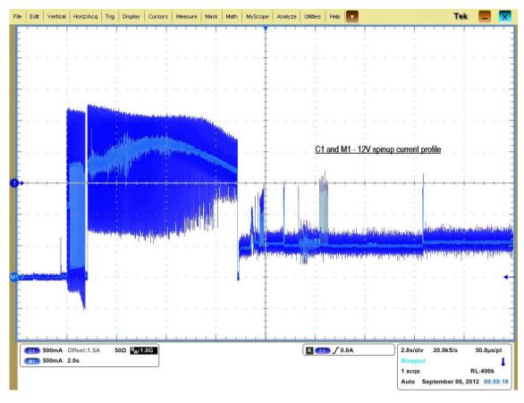
Figure 2. 4TB Typical 12V startup and operation current profile
