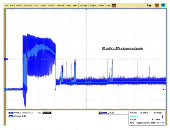
Figure 6. 2TB Typical 12V startup and operation current profile
