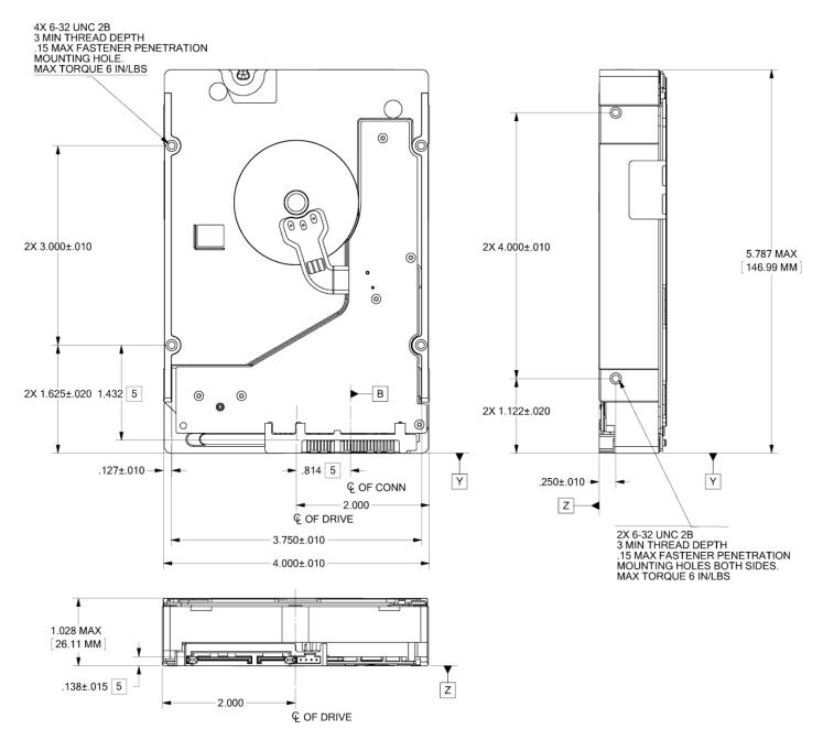
Figure 13. Mounting configuration dimensions (6TB models)
