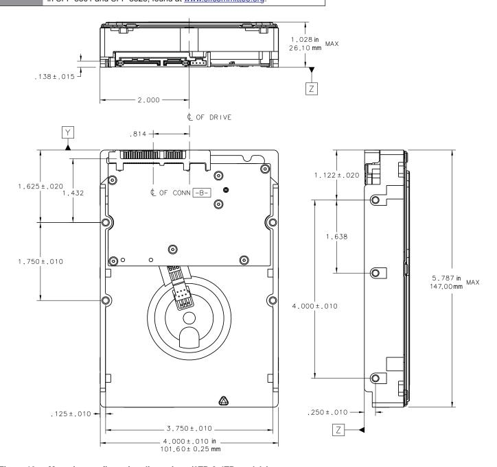
Figure 12. Mounting configuration dimensions (2TB & 4TB models)
