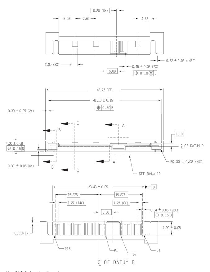
Figure 18. SAS device plug dimensions
