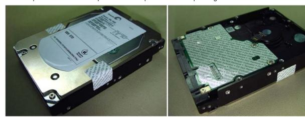
Figure 14. Example of FIPS tamper evidence labels.
