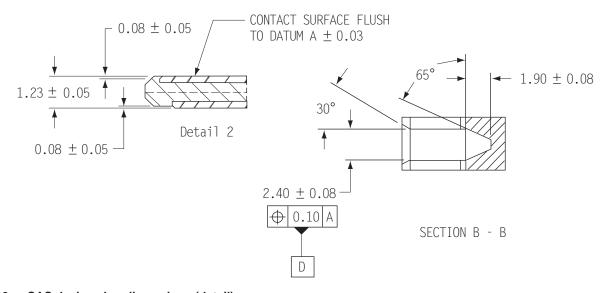
Figure 19. SAS device plug dimensions (detail)
