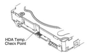
Figure 10. Location of the HDA temperature check point
