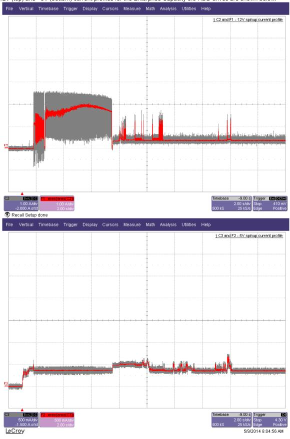
Figure 2. 4TB model current profiles
