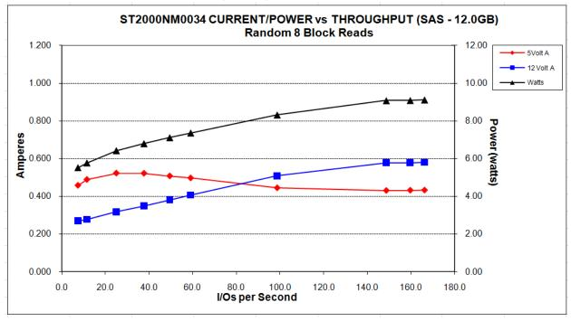
Figure 9. 2TB models (12Gb) DC current and power vs. input/output operations per second
