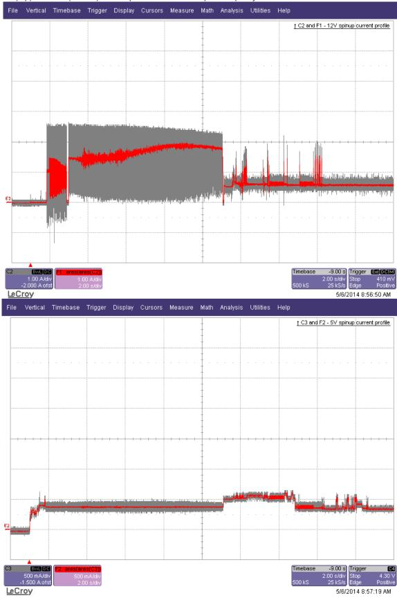
Figure 1. 6TB model current profiles
