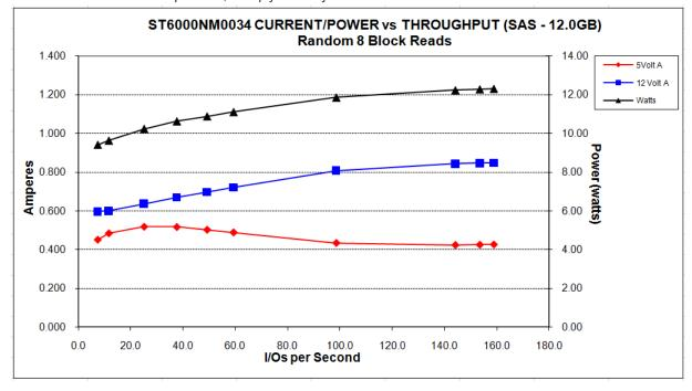
Figure 5. 6TB models (12Gb) DC current and power vs. input/output operations per second
