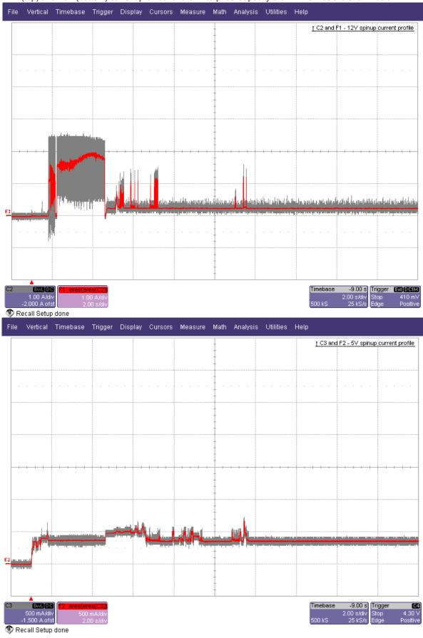
Figure 3. 2TB model current profiles
